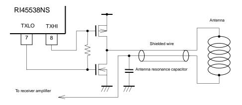
a. When the antenna is driven first.
