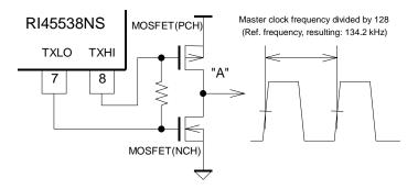
When the IC is in the Receiving Mode, its "TXHI" terminal is fixed at positive level and the "TXLO" at high impedance. As a result, the output terminal "A" of the MOSFET used as an antenna resonance circuit driver is fixed at negative level.
