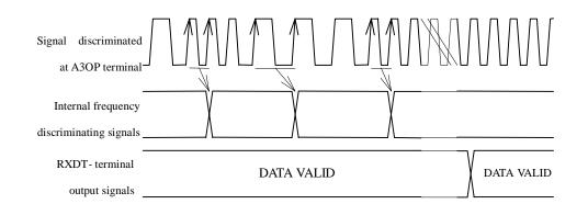
*Note:* For the timing between "A3OP" and "RXDT-" signals, refer to the section describing "Input-Output Specifications".
